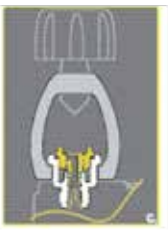
Picture C: Yoke regulator disconnected > regulator closed
